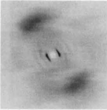
Figure 27. X-ray pattern of a SmC*-elastomer after second uniaxial deformation (reproduced with permission from [83]).
