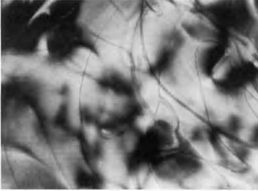
Figure 6. Thin and thick threads in a typical low molecular weight liquid crystal: threaded texture of p -methoxybenzylidene- p - n -butylaniline (MBBA).
