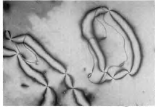
Figure 7. Schlieren texture of terephthalidene-bis-(4- n -butylaniline) (TBBA). Integral nuclei (four brushes) and half-integral nucleus (two brushes).
