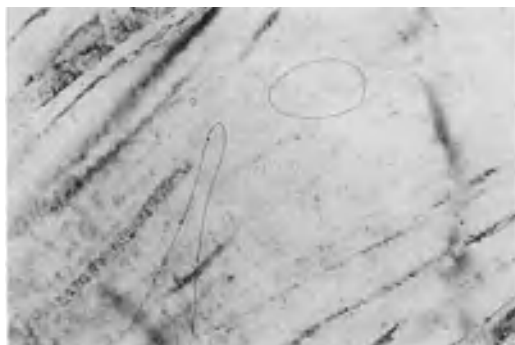
Figure 16. Closed loop viewed between crossed polarizers at 250°C. Copolyester 11 (from [75]).
